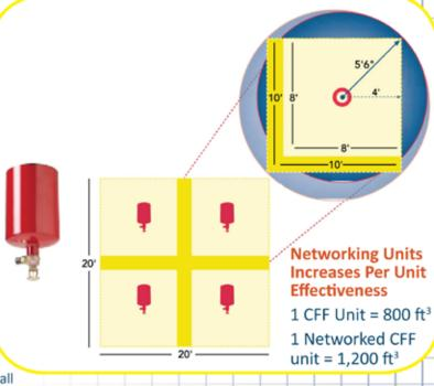
The proprietary, dual-agent, FM-approved CFF 800 units can be networked to provide a total flooding system solution - at a fraction of the cost of piped systems. When two or more units are networked, the extinguishing power increases up to a 10' x 10' area. In this example, four CFF 800 units are networked to protect a 20' x 20' room with up to 12' high ceiling.
